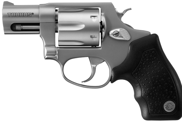
Figure 4.3 Taurus Model 856 in stainless steel. Note the teardrop-shaped recesses in the side of the cylinder. The position of these recesses indicates that this cylinder will have a counter-clockwise rotation. (Image courtesy of Taurus International Manufacturing, Inc.)
